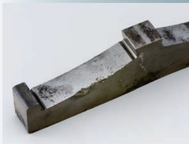
Inner ring breakage
