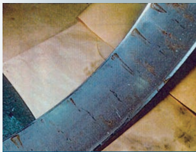
Downtime caused rust
